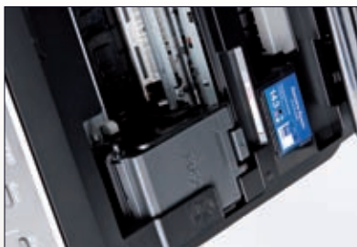
The ink cartridge cradle holds four individual color tanks
